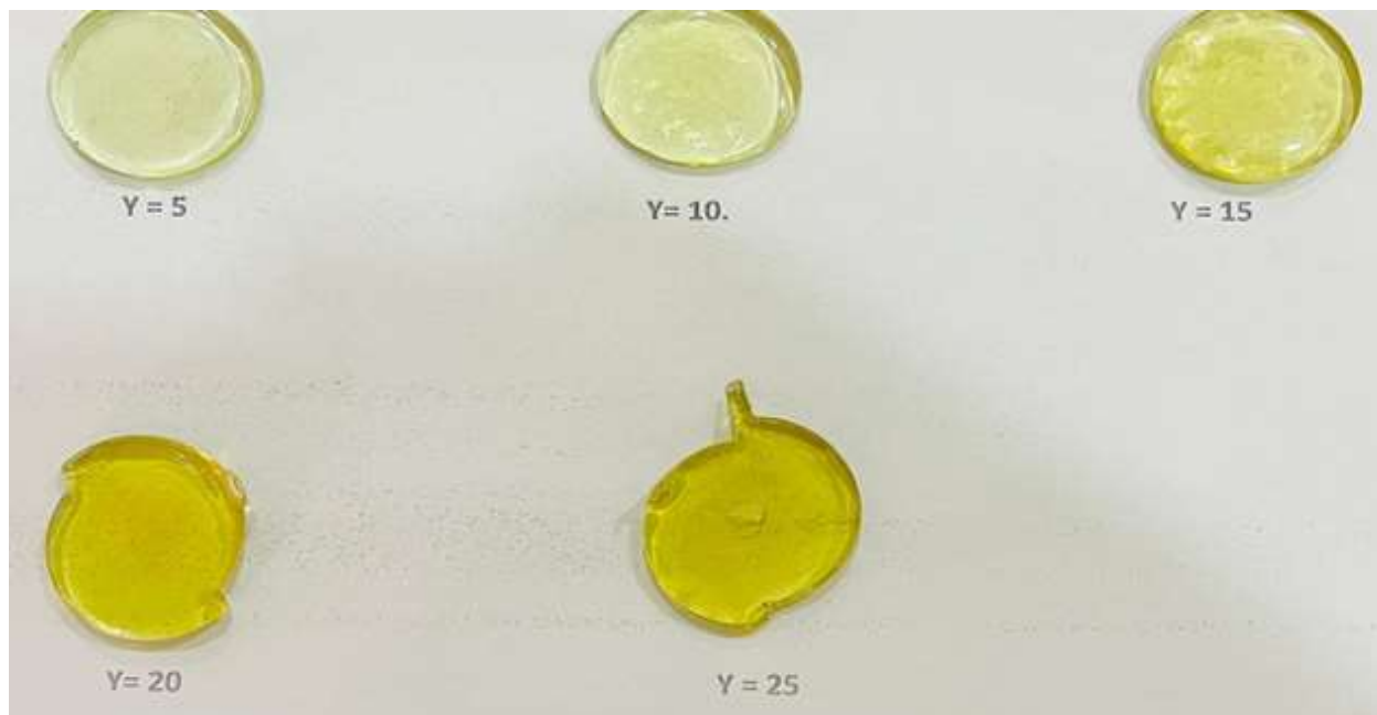
Figure 1. Composition for y = 5, 10, 15, 20 and 25 with empirical formula (100-y)\{85[25(\text{glass sand})+35\text{H}_3\text{BO}_3+40\text{Na}_2\text{CO}_3]+15\text{BaO}\}y[\text{Bi}_2(\text{CO}_3)_2\text{O}_2] of the glass system.
